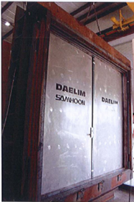
Pretest Photograph of Non-Loaded Side of Door
